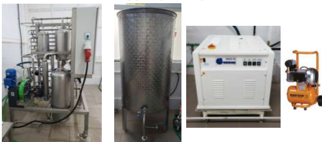
Fig. 8. Direct infusion sterilization installation ISD – main components (ADER 7.5.1.)
